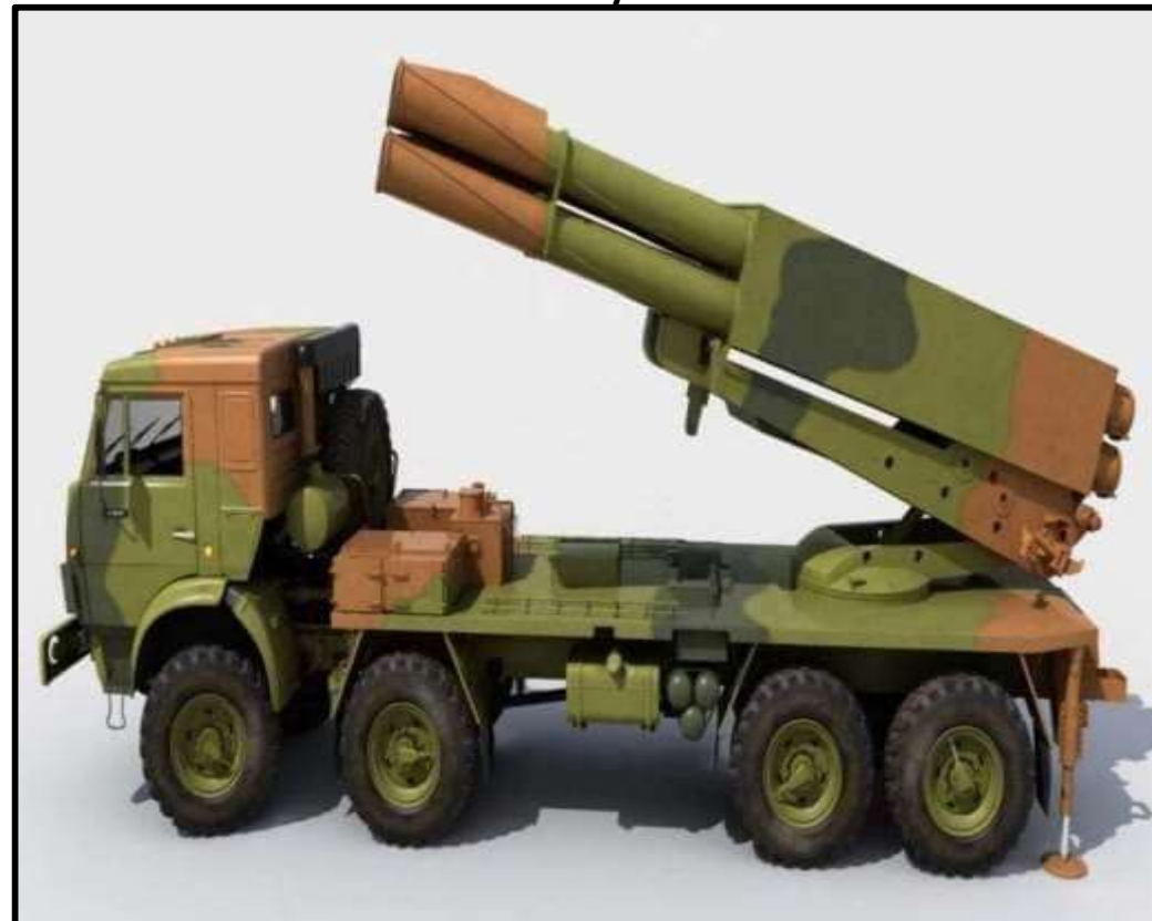
Fabricated components like, Under Frame, Rotating Base Body and Launch Beam Assembly for Rocket Launchers
